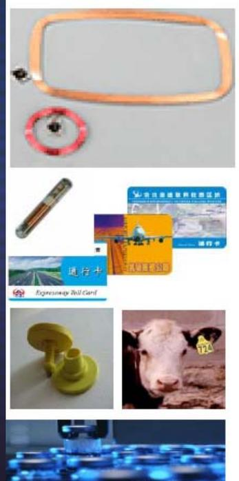
This panel illustrates LF RFID applications. It features a large orange loop antenna, a small red circular antenna, and various identification cards including a Chinese ID card and a 'Greenway 2011 Card'. It also shows a yellow tag on a cow's ear and a hand holding a small device, representing animal tracking and access control.
