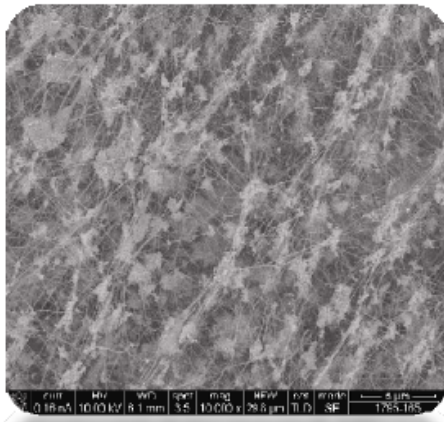
ePTFE media at 10,000x magnification ePTFE滤纸放大10,000x
